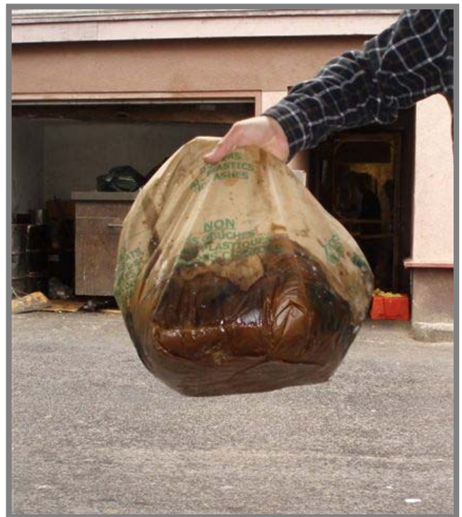
Compostable fiber bags with cellulose polymer lining have proven to be structurally sound when wet although not entirely waterproof. Draining of coffee grounds before disposal would have prevented the saturation shown here.
