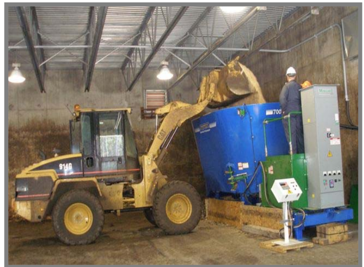
The new vertical mixer accepts a load of woodchips for blending as an amendment during the compost process.
