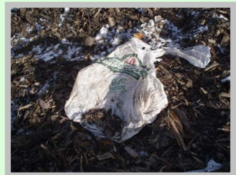
This "100% degradable" bag remains intact after passing through Banff's composting process. It will eventually break down but before it does it may blow around and escape the storage area as litter. Please use only approved bags in compost programmes.
